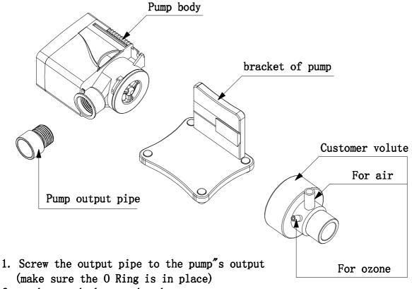
2. push pump body onto bracket
