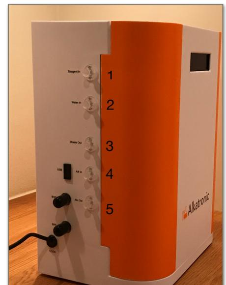
1) Cut the **hose 1.6 mm** in a proper length (if needed). Connect one end to the inlet "**Reagent In (1)**" and the other end to the included long plastic pipe. Put this plastic pipe down into a bottle (not included) which you later will fill up with reagent.
