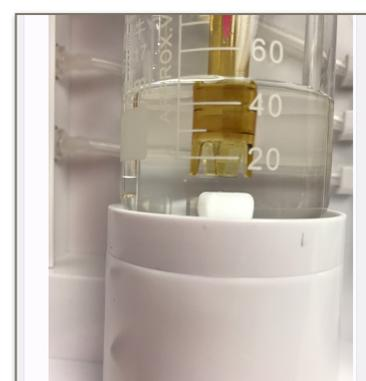
**beaker. Do not place it too close to the bottom, it must never touch the rotating magnetic rod and not touch the glass bottom!** If you of some reasons do not find the rubber ring, use an ordinary rubber band to get the electrode stay in proper position/height.
