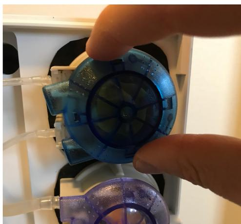
2. Now you have to carefully pull out the hose, and start with pushing the attachment towards you. It should be with no significant resistance, so take
