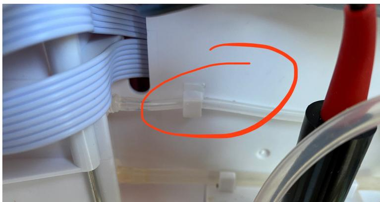
*This is the internal hose that carry the reagent. Do not forget to change this when change hose inside C pump, or if you have issues with many black dots.*
