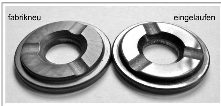
Fig. 2: Bearing stright from factory and following run-in phase
